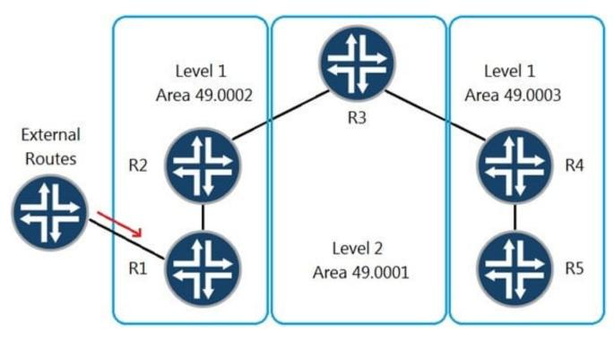
Referring to the exhibit, external routes are being received at R1. These routes must appear on R5. Which action will produce this result?
