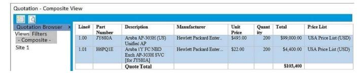
A hotel needs a wireless solution. The architect has selected 303H Series, controlled by a local MC, as the best choice. The hotel plans to have the APs installed in the existing wall boxes which have one Ethernet port each. The architect has created to BOM shown in the exhibit. (Note that this portion of the BOM does not include the MC, which is not part of this question.)
