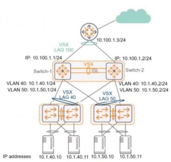
Switch-1, Switch-2, and the router run OSPF on LAG 100, which is a Layer 3 LAG. Does this correctly explain how to control how core-to-access traffic Is forwarded? Solution: To reduce the amount of traffic sent over the ISL between Switch-1 and Switch-2. enable Equal Cost Multi Path (ECMP) on both Switch-1 and Switch-2.
