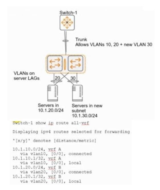
You are adding a VLAN 30, subnet 10.0.30.0/24 to the network shown in the exhibit. (This network is simplified to just the relevant switches for this item.) This subnet belongs in VRF A, and you have added a Layer 3 VLAN 30 interface
