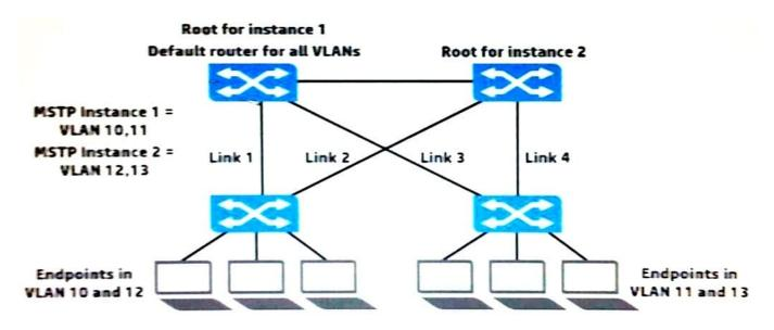
The network administrator is setting up Multiple Spanning Tree Protocol (MSTP) with the settings shown in the exhibit. All the switches are in the same region. The administrator has requested help determining which VLANs each switch-toswitch link should carry. What is a recommendation for this topology?
