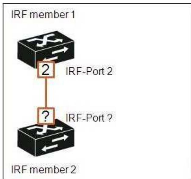
An IRF-stack is being built using HP A5800 switches, and IRF member 1 will be connected to IRF member 2 using IRF-port 2. Which IRF-port should it be connected to?
