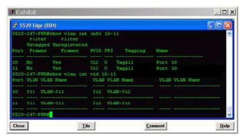
Reference the output of the two show commandsfrom an edge Ethemet Routing Switch 5520-24T-PWRshown in the exhibit. Anuntagged frame arrives on port 10, which is configured as an accessport. To which VLAN will the packet be forwarded?
