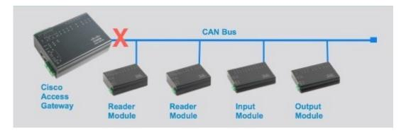
In the event of a loss of connectivity from the Cisco Access Gateway to the expansion modules on the CAN bus, with DC power still connected, what will happen if an access card was presented to a card reader that is connected to one of the Reader Modules?
