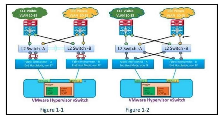
Refer to the exhibit. Which option describes Cisco Unified CCE on the UCS B Fabric Interconnection pair to the upstream network connectivity?
