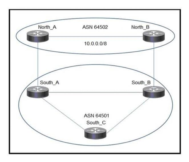
A network engineer sets up a multihoming eBGP topology where multiple Autonomous Systems connect to ASN 64501. The engineer wants to block all the routes coming from ASN 64502 but allow all the others. For that purpose, the
