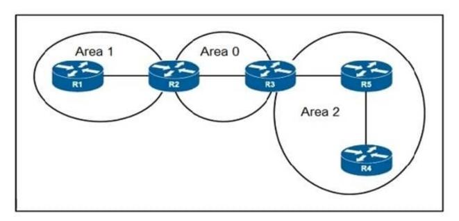
A network engineer applied configuration on R5 to summarize all OSPF routes, but R4 is still receiving specific routes from R5. The engineer has confirmed that both R5 and R4 routers are configured with correct summarization
